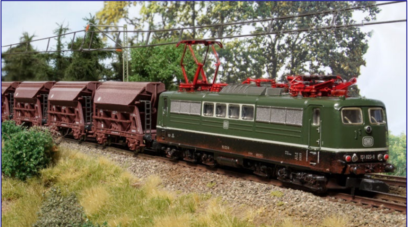
The five-pole motor helps 151 023-9 from the starter set to deliver better driving characteristics compared to its predecessor. Here, it is on the move with a goods train transporting fertiliser for agriculture.
