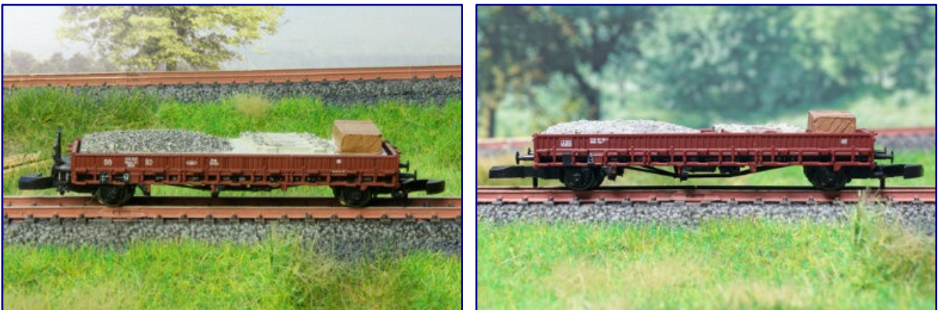
This comparison of the factory condition (left) and the reworked insert (right) is intended to enable a comparison: The load now sits much lower in the wagon and no longer looks over the edge.
