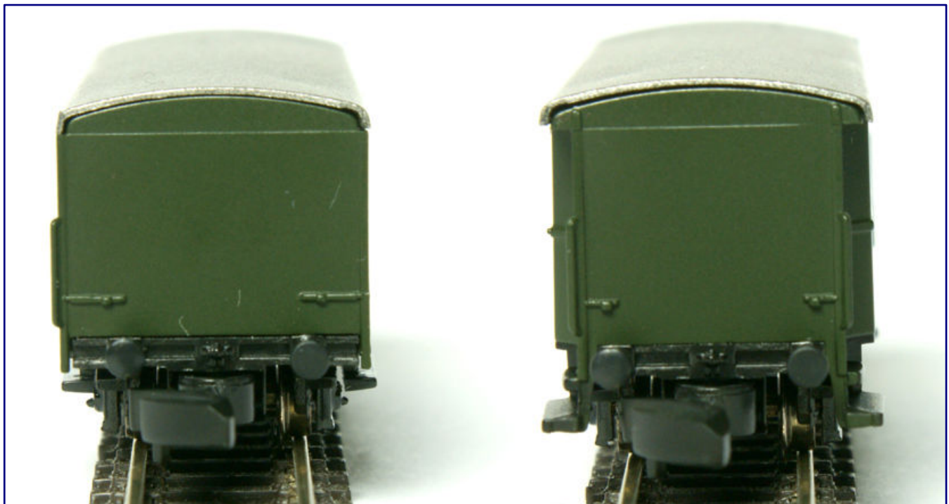
Both front sides no longer show ladders and also no holders for upper carriage lanterns. This corresponds to the upgrades carried out on the prototypes around 1959.
