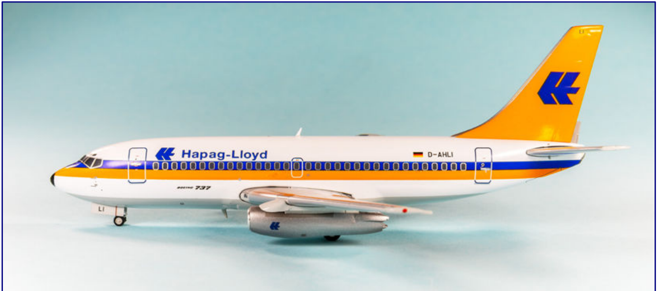
The external distinguishing feature of the Boeing 737-200 Advanced was the elongated shape of the engines under the wings, which can also be seen immediately on the model. Photo: Oleksiy Mark
