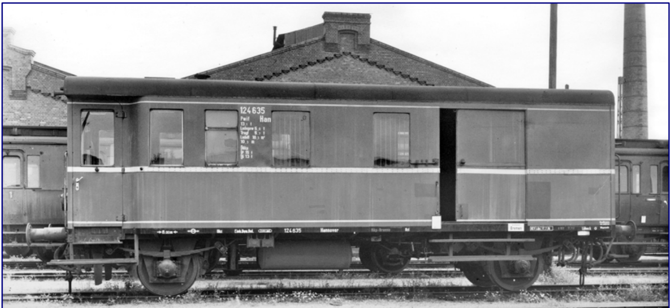
The purple red Pwif 41/52 driving trailer with the road number 124 635 Han, photographed in 1956, was converted by the DB four years earlier. It shows a possible type of shape of the new product, provided that this option was also taken into account in the tooling. Photo: Günter Scheingraber, Railway Foundation
